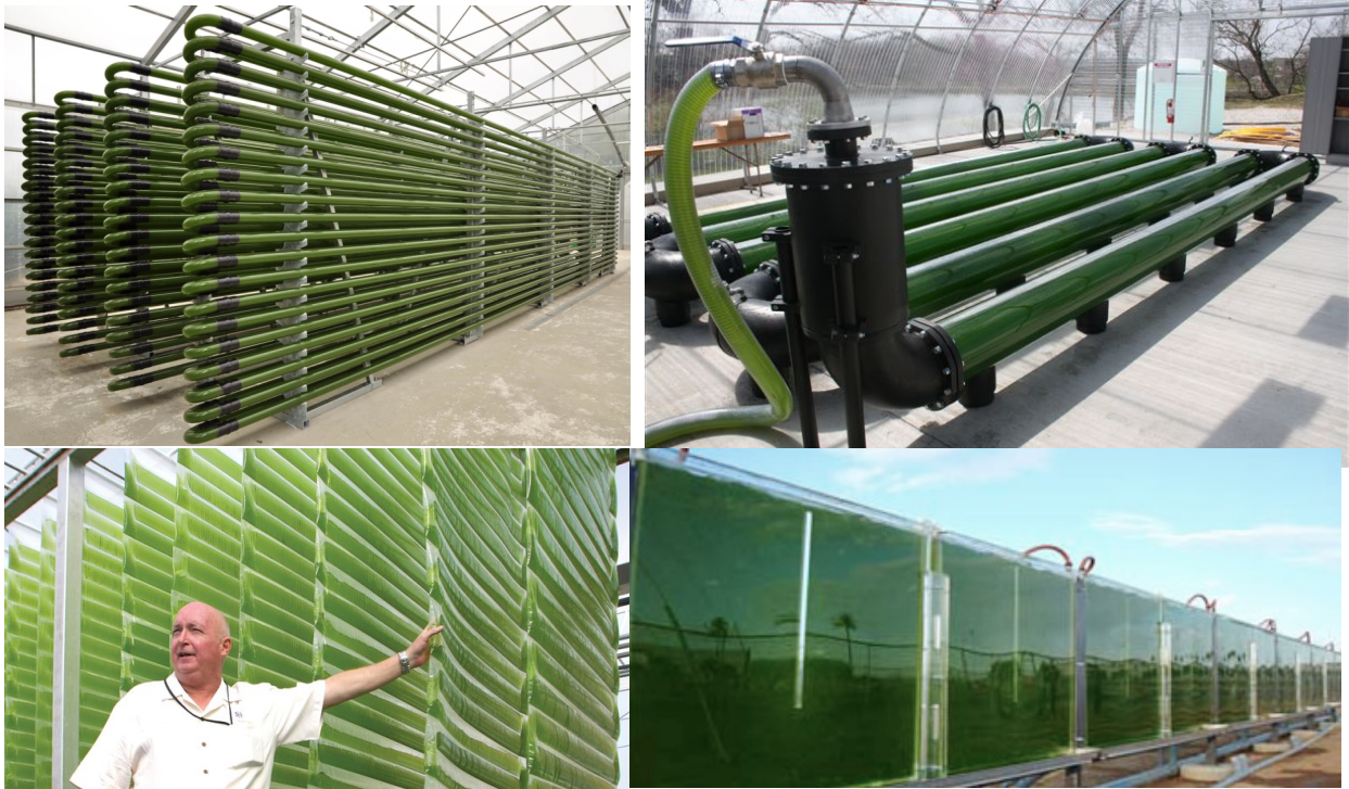
Figure 3: Examples of closed systems (photobioreactors) for growing algae.
