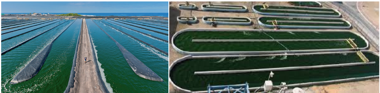
Figure 4: Examples of open systems for growing algae. The systems in these photos are called 'raceway ponds.'
